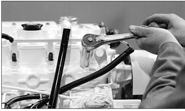
Figure 18: Reinstall injector. Torque to proper tightness.
