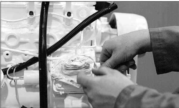
Figure 13: Cover lines, inlets and injection pump outlets.
