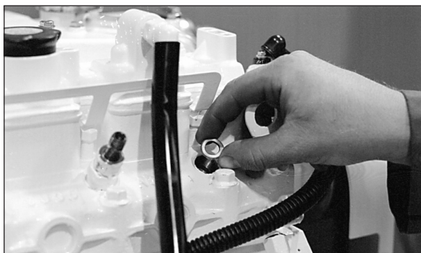
Figure 17: Remove and replace copper sealing washer.
