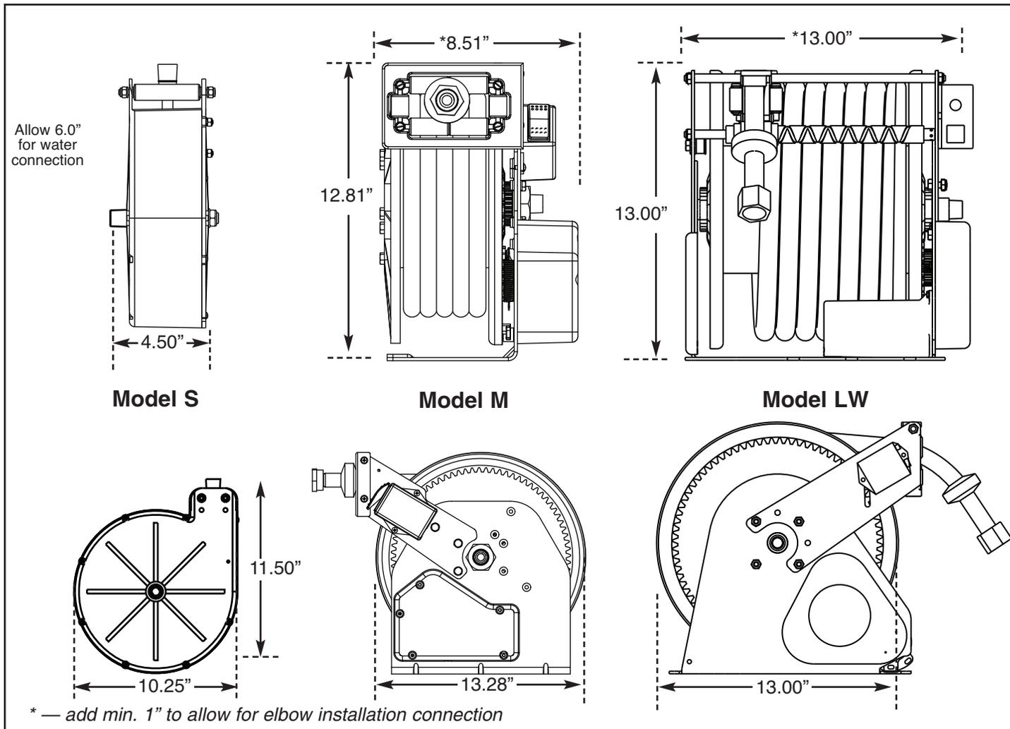
**Hosemaster - Model S** (Spring hose retraction, hose ID = 0.330 inch, 8 to 16 feet long. Sprayer and receptacle not included - unless specified)
