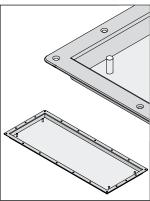
Extremely stable mounting system with fixed bolts for installation on deck cutouts.
