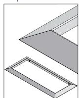
Ramp frame to cover the deck-rails when built »on deck«.
