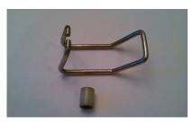
2. The only thing preventing the bailer from dropping out of the bottom is the bent stopper tab at the rear of the bailer slide. Carefully use vise grips or pliers to bend it straight.
