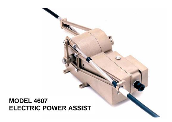
The purpose of the 4607 is to provide a power assist for hard to move push pull cable systems. It can provide a maximum torque of 120 in-lbs.
