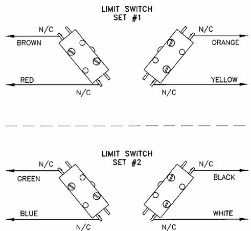
**Fig. 2** Wiring diagram of micro switches
