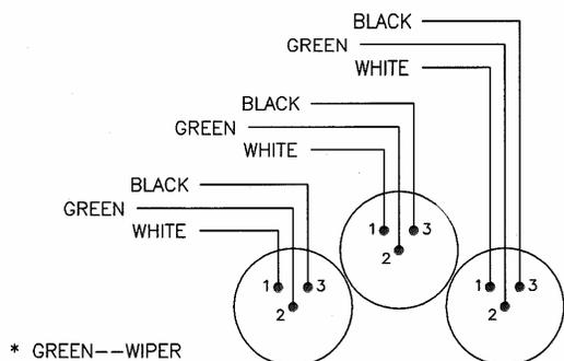
**Fig. 1** Wiring diagram of potentiometers
