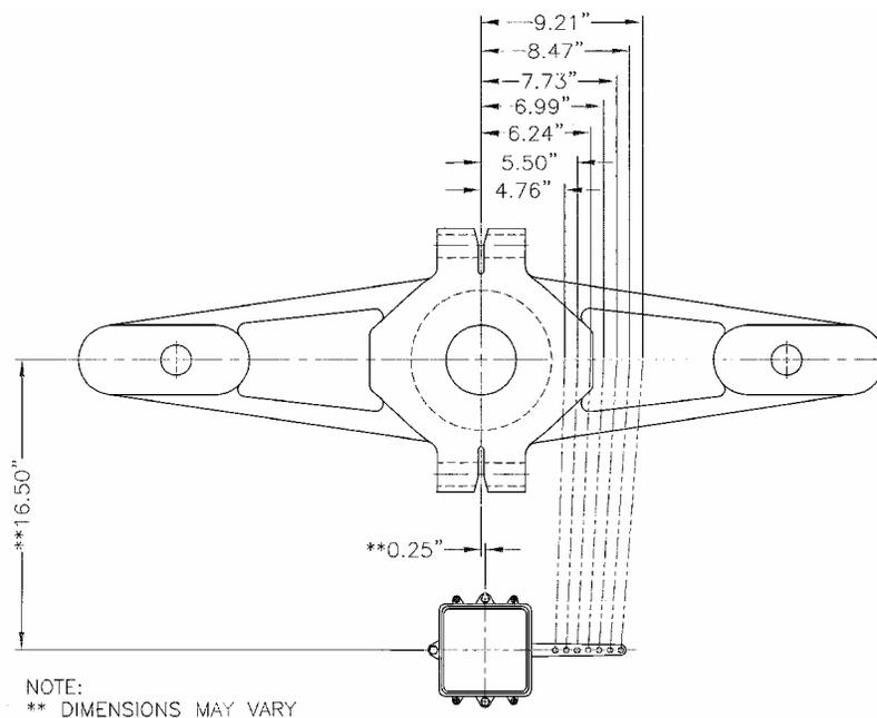
Diagram 4: Example of installation for rudder movement 35°-0-35°
