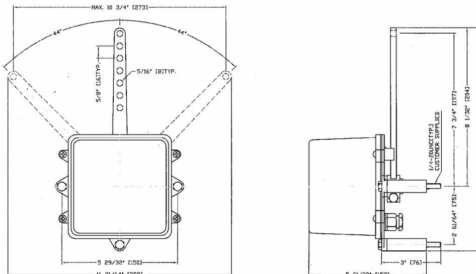
**Diagram 3:** Dimensions of 7174 rudder angle feedback unit
