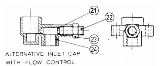
✦Alternative inlet cap with flow control (item 24) can be used to replace item 18.
