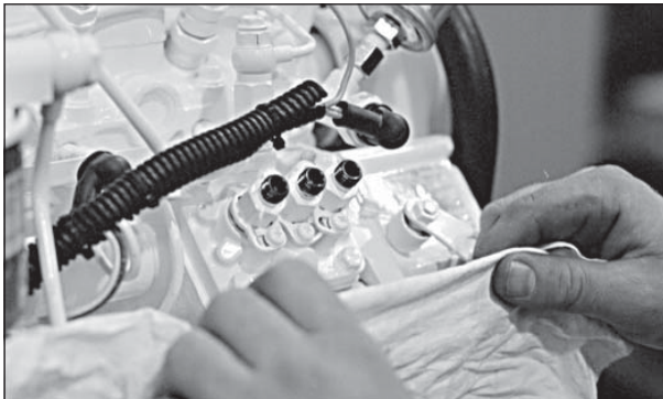
Figure 15: Cover lines, inlets and injection pump outlets.
