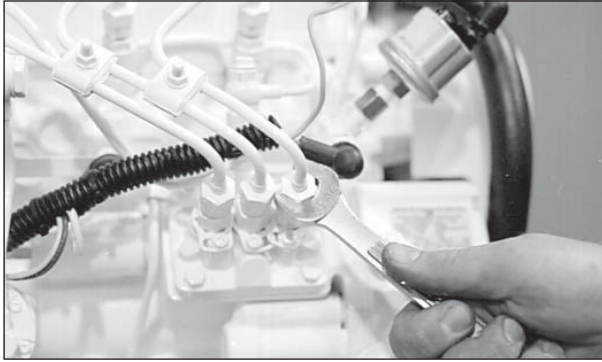
Figure 13: Remove delivery line flare nuts.
