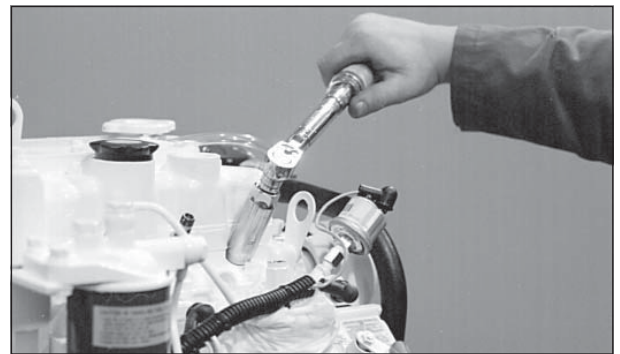
Figure 20: Reinstall injector. Torque to proper tightness.
