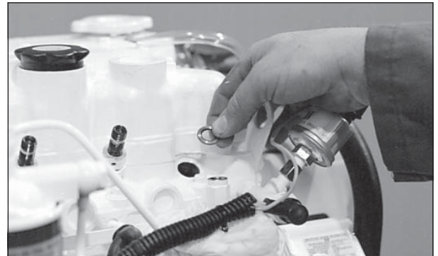
Figure 19: Remove and replace copper sealing washer.
