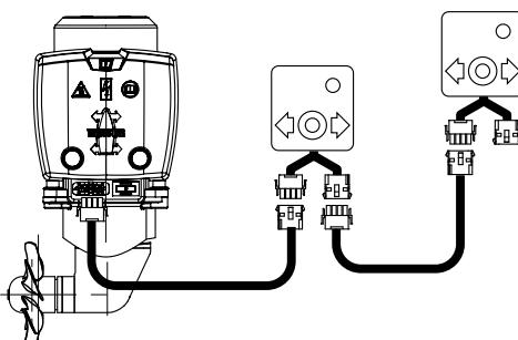
If it is found during test running that the thrust direction does not correspond with the direction switch on the control panel then the blue (no. 1) and the white (no. 4) wires on the relay must be interchanged.
