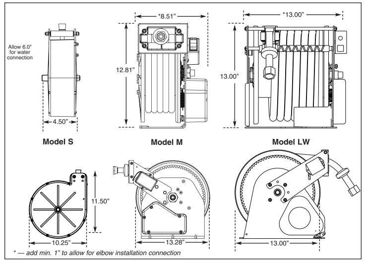
Hosemaster - Model S (Spring hose retraction, hose ID = 0.330 inch, 8 to 16 feet long. Sprayer and receptacle not included - unless specified)
