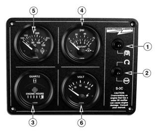
Figure 3-B: Series 3 Generator Control Panel
