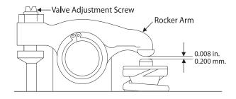
Figure 7: Valve Adjustment
