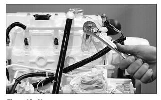
Figure 15: Unscrew injector.
