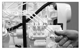
Figure 10: Remove delivery line flare nuts.
