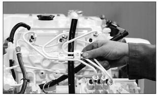
Figure 11: Remove delivery lines.
