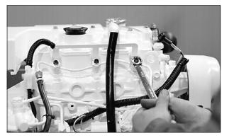
Figure 13: Remove return line nuts.
